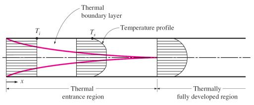
The region of flow over which the thermal boundary layer develops and reaches the tube center is called the **thermal entrance region**, and the length of this region is called the **thermal entry length**  $L_t$ .
