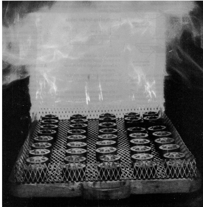
Parts to be carburized in a nitrogen-methanol carburizing atmosphere
