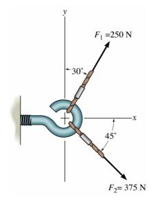
\*2-4. Determine the magnitude of the resultant force  $\mathbf{F}_R = \mathbf{F}_1 + \mathbf{F}_2$  and its direction, measured clockwise from the positive u axis.
