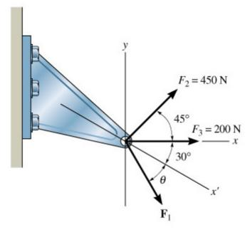
2-37. Determine the magnitude and direction  $\theta$  of  $\mathbf{F}_1$  so that the resultant force is directed vertically upward and has a magnitude of 800 N.
