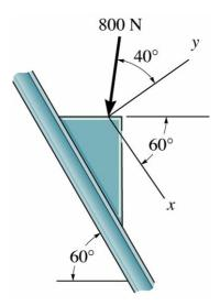
\*2-32. Determine the magnitude of the resultant force and its direction, measured clockwise from the positive x axis.
