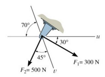
2-5. Resolve the force  $F_1$  into components acting along the u and v axes and determine the magnitudes of the components.
