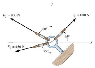
**2-3.** Determine the magnitude of the resultant force  $\mathbf{F}_R = \mathbf{F}_1 + \mathbf{F}_2$  and its direction, measured counterclockwise from the positive x axis.
