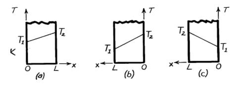
(14) Consider a large plane wall of thickness L  $\_$  0.2 m, thermal conductivity k  $=1.2 \text{ W/m} \cdot \text{K}$ , and surface area A = 15 m2. The two sides of the wall are maintained at constant temperatures of T1  $= 120^{\circ}\text{C}$  and T2  $= 50^{\circ}\text{C}$ , respectively. Determine (a) the variation of temperature within the wall and the value of temperature at x = 0.1 m and (b) the rate of heat conduction through the wall under steady conditions.
